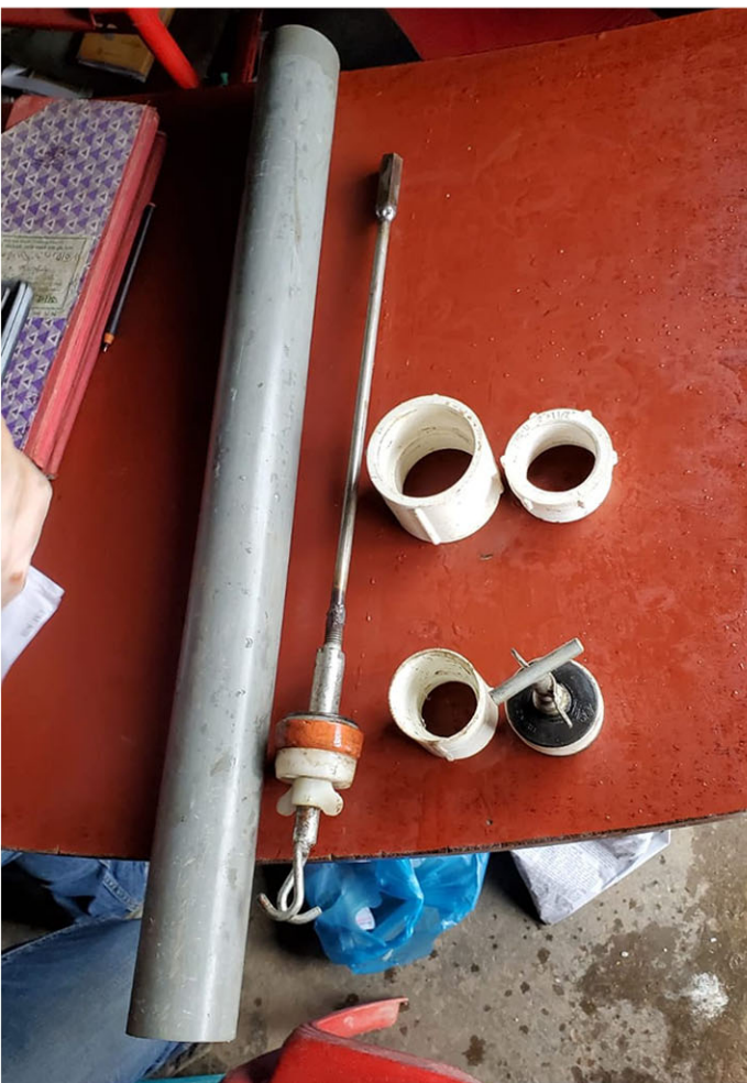
New well pump cylinder
